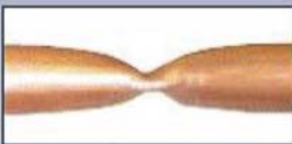
Wheeler-Rex Shut-Off tools effectively compress soft copper tubing to shut off water flow.
